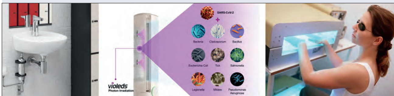
A point-of-use water purification system (left). A list of viruses and bacteria that the air-conditioning systems with incorporated UVC LED array can mitigate (middle). A UVB LED based psoriasis treatment system (right).
