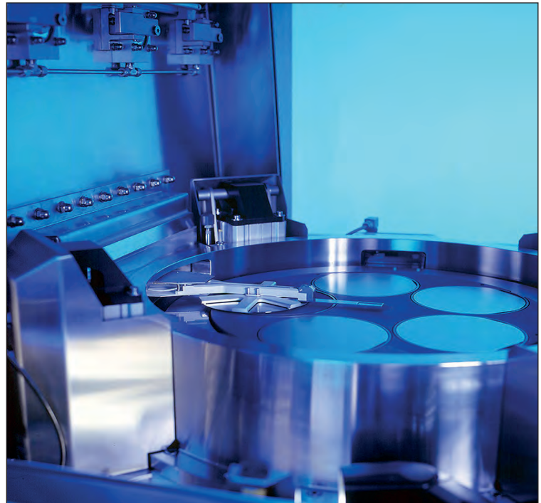
Figure 8. View in an AIX 2600 G3 Planetary Reactor equipped with a wafer loader as delivered in 1996.
