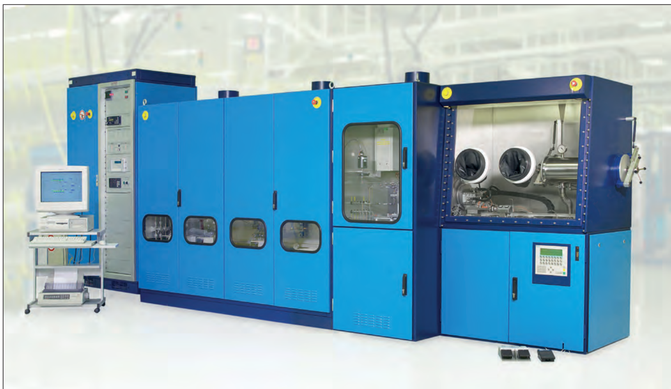
Figure 4. Standard lamp-heated Aixtron 200/4 system with the typical blue colour, glove box and computer control. This reactor was used primary for growing GaAs- and InP-based material systems. One wafer up to 4 inch fits into the reactor.
