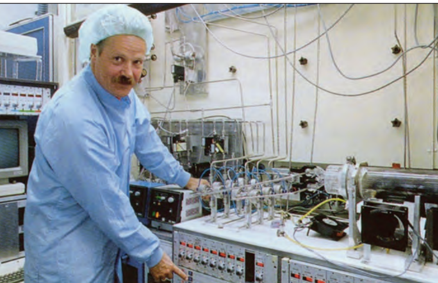
Figure 3. Holger Jürgensen, co-founder of Aixtron, operating one of the company's first prototype reactors, used at that time for the growth of InP materials at RWTH Aachen University. The early work was undertaken in co-operation with D. Grützmacher, today professor at FZ Jülich. The image shows the quartz reactor, early versions of the vent run system and so-called read out boxes to set the mass-flow control (MFC) readings. Fans under the reactor were switched on in the cool down phase to decrease cool down time and increase productivity. Picture from late 1980s.
