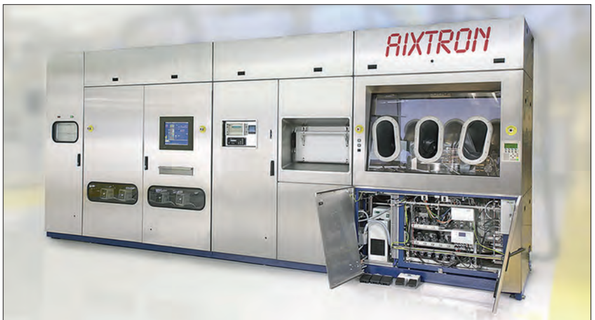
Figure 7. The Planetary Reactor in the integrated concept design. Beside productivity improvements, the stainless steel outlook approaches silicon fab style.
