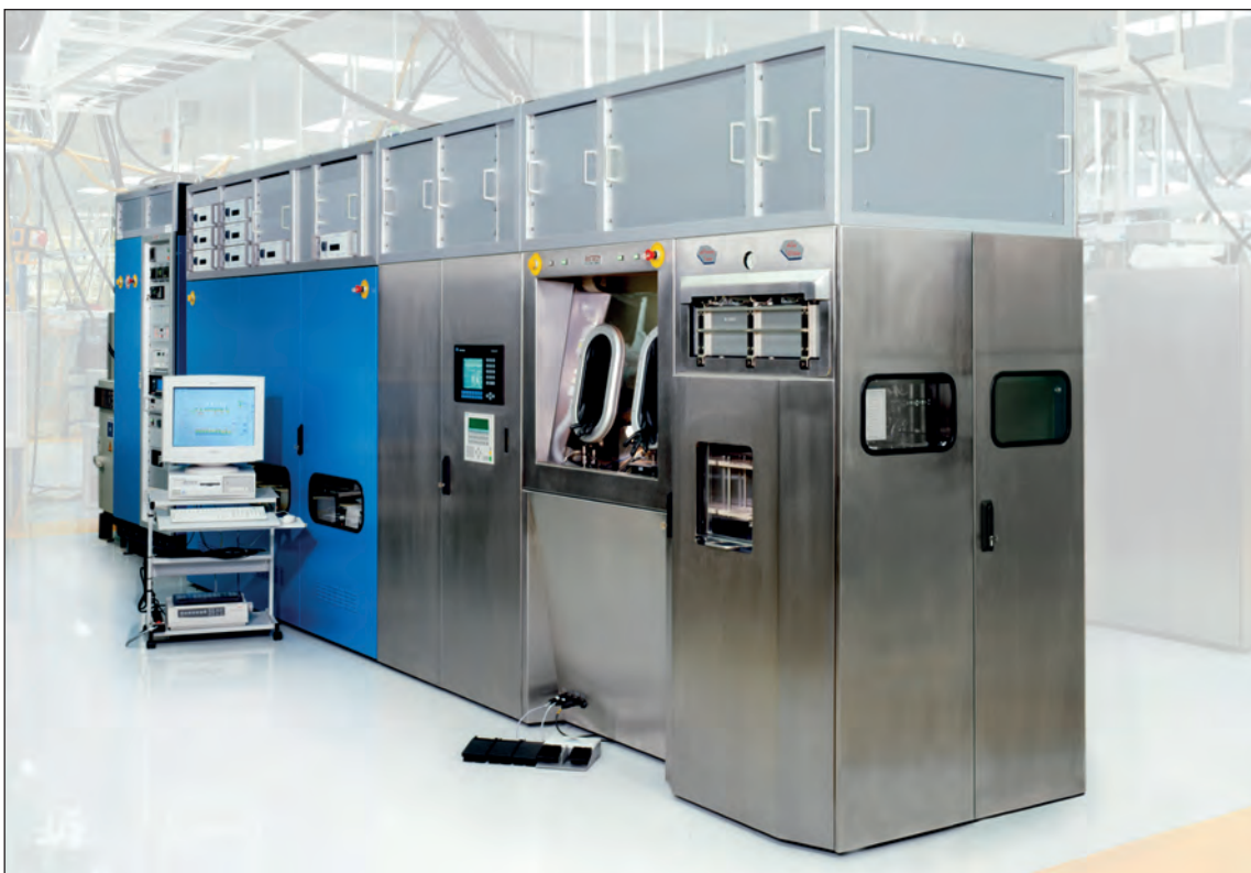
Figure 9. An early Planetary Reactor.
